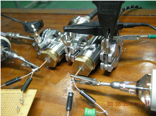
Fig. 4. Experimental setup for the two spark gaps system.
