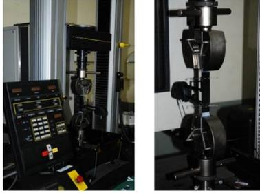
Fig. 6 Experimental set-up for tensile test.
