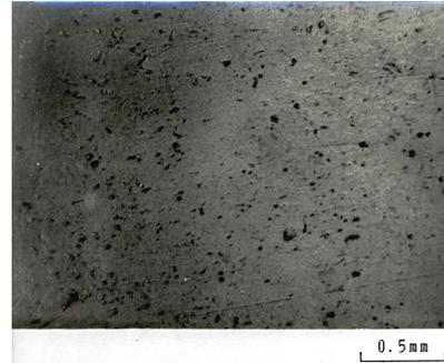
Fig. 6 Surface of moldings having coating layer.
