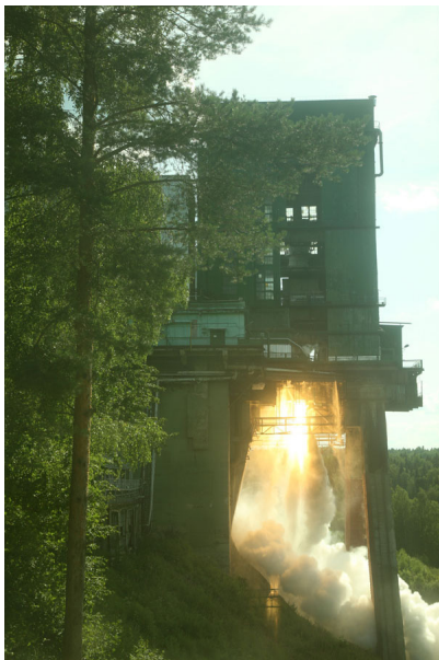
Fig. 4 Angara firing test (from Russian space Web, credit: Khrunichev)
