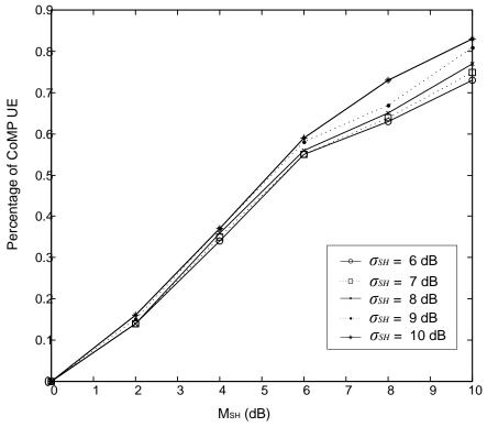
Fig. 9. Percentage of CoMP UE versus  $M_{SH}$  for different values of  $\sigma_{SH}$
