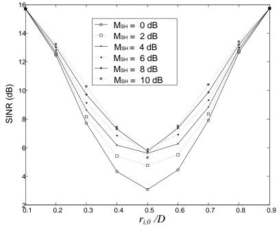
**Fig. 5.** SINR depending on distance  $r_{i,0}$  /*D* (m = 4,  $\sigma_{SH} = 8$  dB, and  $\varepsilon = 0.05$ )
