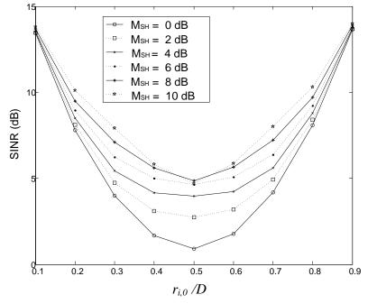
**Fig. 4**. SINR depending on distance  $r_{i,0}$  /*D* (m = 3,  $\sigma_{SH} = 8$  dB, and  $\varepsilon = 0.05$ )
