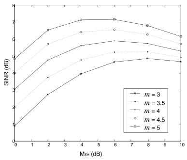
**Fig. 7.** SINR versus  $M_{SH}$  for different values of pathloss exponent *m* (distance  $r_{i,0}/D = 0.5$ )
