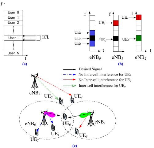
**Fig. 3**. Assumption for interference analysis (**a**) Resource allocation by semi-static scheduler (**b**) Example of user allocation in eNBs and (**c**) Multi-point reception and inter-cell interference model
