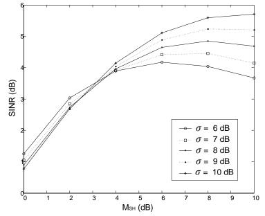
**Fig. 8.** SINR versus  $M_{SH}$  for different values of  $\sigma_{SH}$  (distance  $r_{i,0} / D = 0.5$ )
