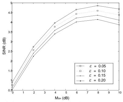
**Fig. 6**. SINR versus  $M_{SH}$  for different values of  $\varepsilon$  (distance  $r_{i,0} / D = 0.5$ )
