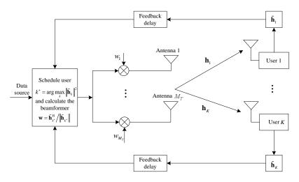
Fig. 1. System model of the M-TMRC scheme with outdated feedback.
