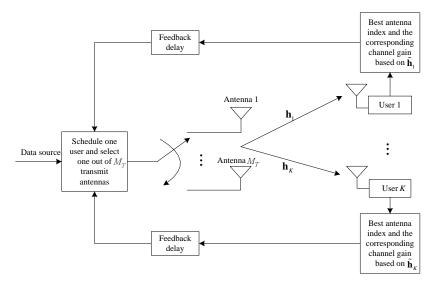
Fig. 2. System model of the M-TAS scheme with outdated feedback.
