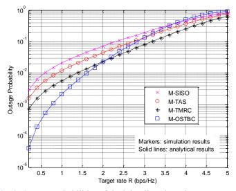
Fig. 8. Outage probabilities of the joint diversity schemes vs. R, with  $\overline{\gamma} = 10 \text{ dB}, K = 10, M_T = 2 \text{ and } \rho = 0.7$ .
