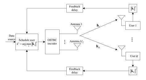
Fig. 3. System model of the M-OSTBC scheme with outdated feedback.
