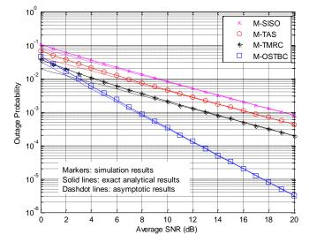
Fig. 4. Outage probabilities of the joint diversity schemes vs.  $\overline{\gamma}$ , with  $K = 10, M_T = 2, \rho = 0.7$  and R = 0.5 bps/Hz.
