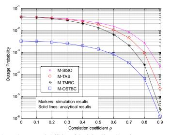
Fig. 7. Outage probabilities of the joint diversity schemes vs.  $\rho$ , with  $\overline{\gamma} = 10 \text{ dB}$ , K = 10,  $M_{\tau} = 2 \text{ and } R = 0.5 \text{ bps/Hz}$ .
