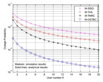
Fig. 5. Outage probabilities of the joint diversity schemes vs. *K* , with  $\overline{\gamma} = 10 \text{ dB}, M_T = 2, \rho = 0.7 \text{ and } R = 0.5 \text{ bps/Hz}$ .
