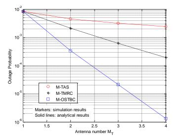
Fig. 6. Outage probabilities of the joint diversity schemes vs.  $M_T$ , with  $\overline{\gamma} = 10$  dB, K = 10,  $\rho = 0.7$  and R = 0.5 bps/Hz.
