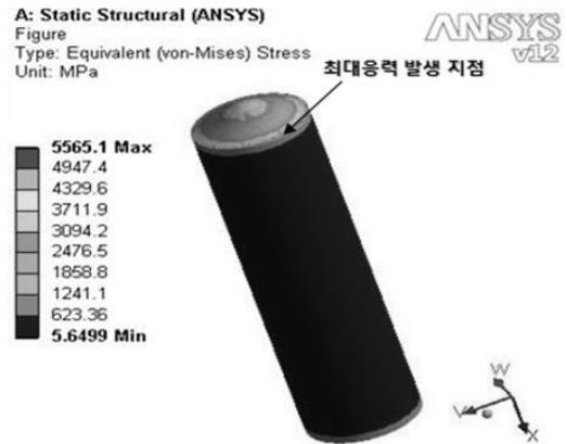
Fig. 14. Simulation of stress distribution during an internal explosion of D cylinder structure.
