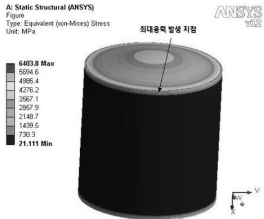
Fig. 13. Simulation of stress distribution during an internal explosion of C cylinder structure.
