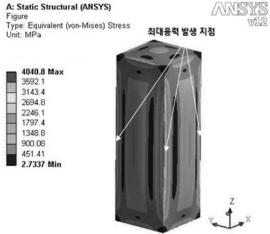
Fig. 9. Simulation of stress distribution during an internal explosion of A rectangle structure.
