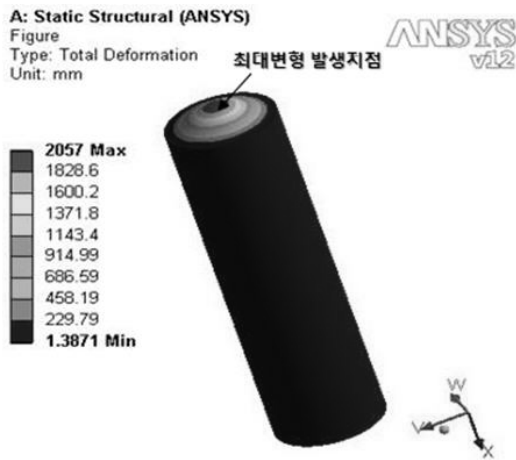
Fig. 12. Simulation of deforming during an internal explosion of D cylinder structure.
