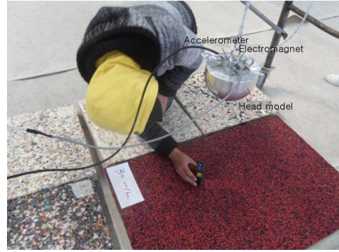
Figure 6. Picture of critical fall height test
