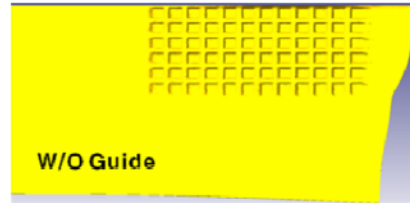
(b) Deformed shape(w/o guide, after 0.8° rotation of rolls)
