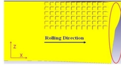
Fig. 6 Deformed shape at intermediate stage of the R2R forming
