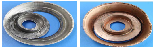
Fig. 16 Failure result of 2nd forming
