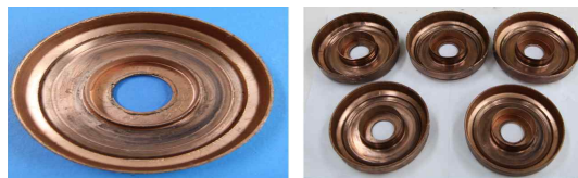
Fig. 17 Succeeded in 2nd forming brass model
