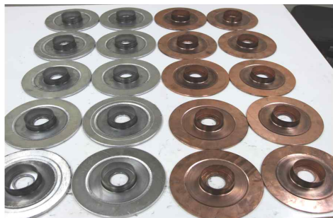
Fig. 15 Succeeded in 1st forming Al and brass model (Speed 400rpm, feed 16mm/min)
