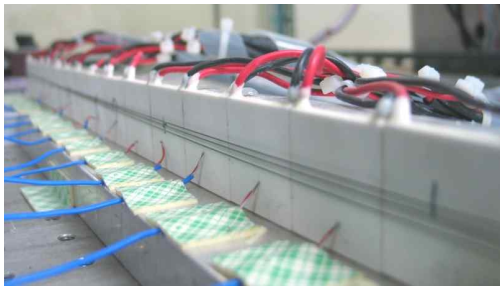
(b) SMA wire segmented by TEM Fig. 2 Segmented SMA actuator
