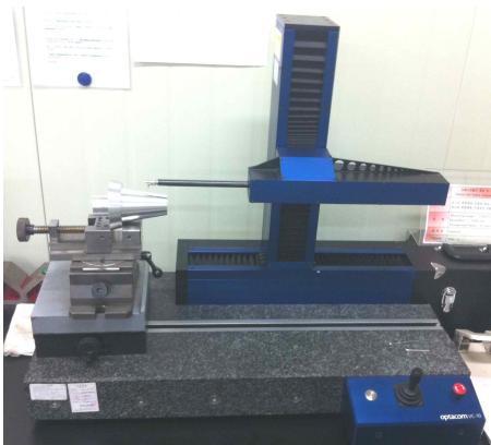
Fig. 4 Photograph of surface roughness measuring
