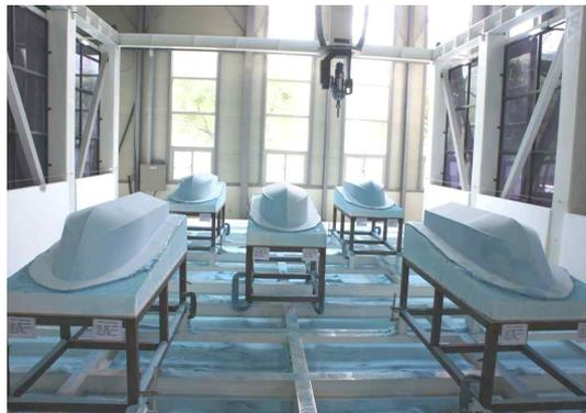
Fig. 7 Finish machining of resin
