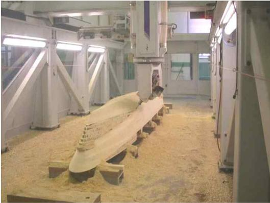
Fig. 2 Manufacturing process(5-axis machine)
