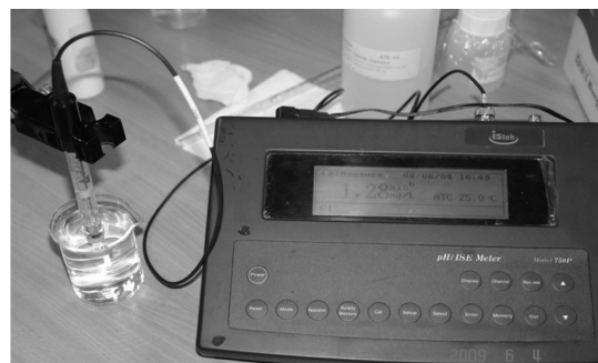
Fig. 4. Measurement of chloride ion concentration.
