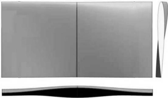
Fig. 1 Top, side and front view of the 3D twisted hydrofoil
