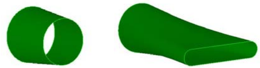
a) Circular nozzle b) Rectangular nozzle
