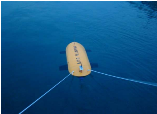
Fig. 9. Free running test in towing tank
