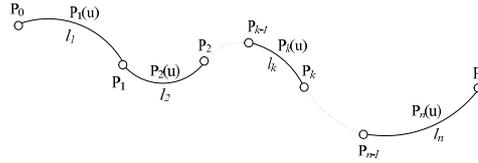
Fig. 1 Cubic spline interpolating n+1 data points
