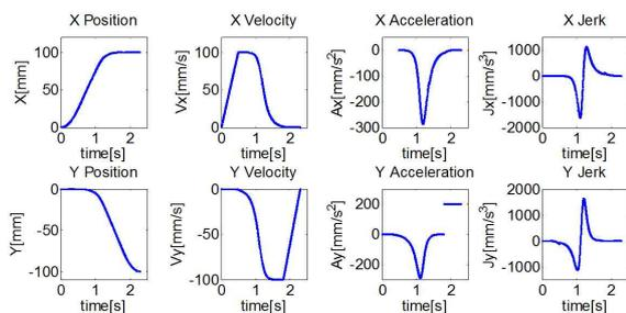
Fig. 6 P, V, A, J for X, Y coordinates for case 3
