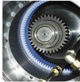
Fig. 2 Gear honing manufacturing
