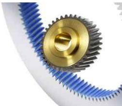
Fig. 1 Producing of hone by diamond dressing gear
