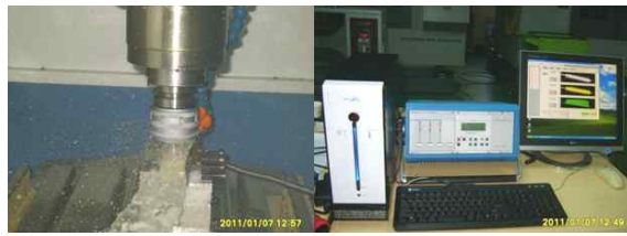
Fig. 3 Cutting force measurement using dynamometer
