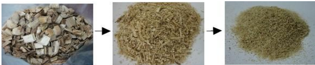
[Fig 1] Preparation of Wasted Corn Stalk for Experiment. (from left : cut, 1st Pulverization, 2nd Pulverization)
