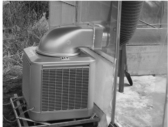
Fig. 2. An integrated fan and pad system for use in experiment.
