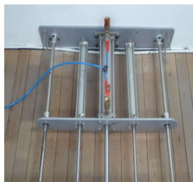
Fig. 1 Pneumatic actuator for fall guidance
