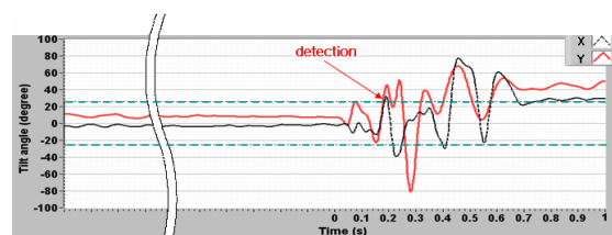
Fig. 5(b) Tilt angle during forward fall
