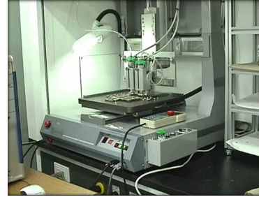
Fig. 6 Robotic dispensing system
