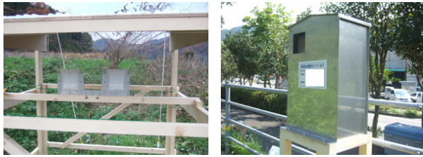
(a) JIS style (b) Toyun style Figure 1. Existing incoming salt collector [8]
