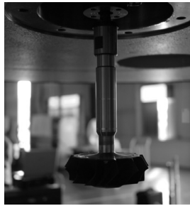
Fig. 16 Assembly of turbine system for spin test
