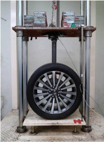
Fig. 3 Experimental apparatus for vertical tire stiffness test
