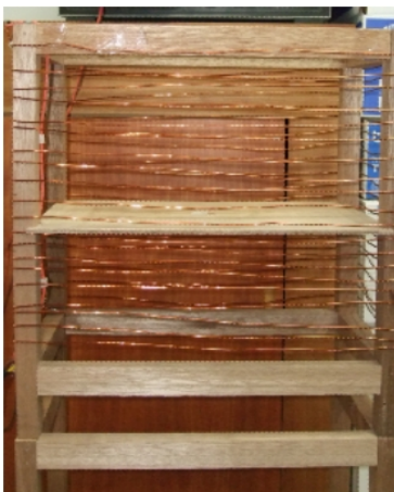
Fig. 2. Magnetic field generating coil wound on a wooden frame. A small resonating capacitor for L-C series resonance is hidden and not shown in the figure.
