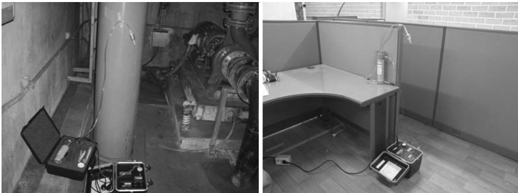
Fig. 1. Monitoring of radon concentration at each locations using RAD-7 system.
