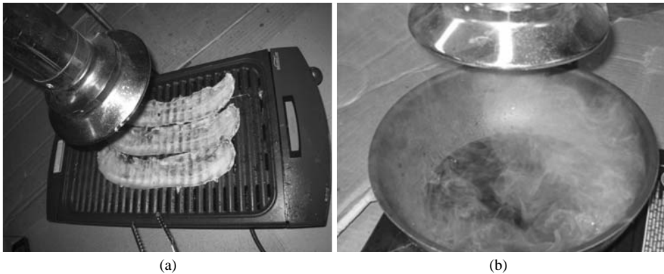
Fig. 1. Meat cooking method (a) and oil mist generation for long time test (b).
