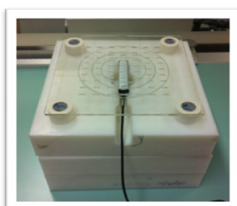
Fig. 4. 20 cm thickness acrylic phantom(25 cm × 25 cm) and multifunction meter
