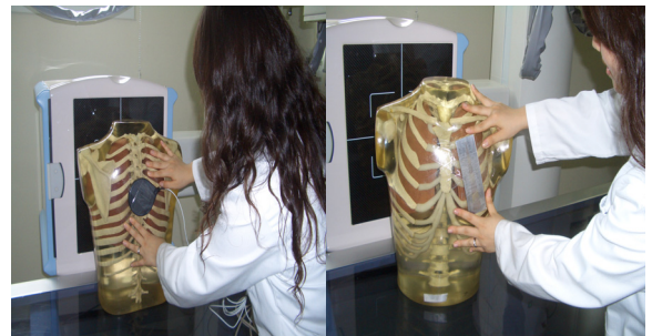
Fig. 2. Install the Ion-chamber and the Spatial resolution chart
