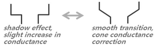
Figure 7. Two methods for connecting two components with different cross-sections.
