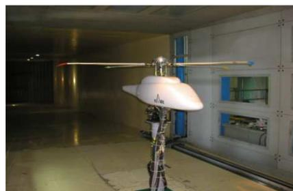
Fig. 3 GSRTS in Sub-sonic Wind Tunnel of KARI
