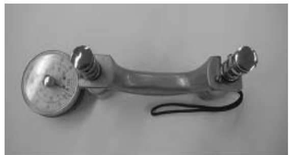
Fig 1. Hydraulic hand dynamometer (Jamar 5030J1, USA)
