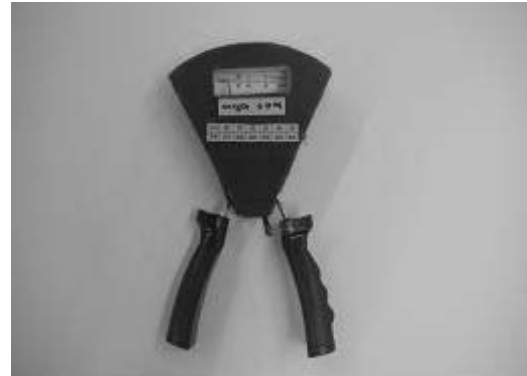
Fig 4. Developing a prototype capable of measuring muscle strength age
