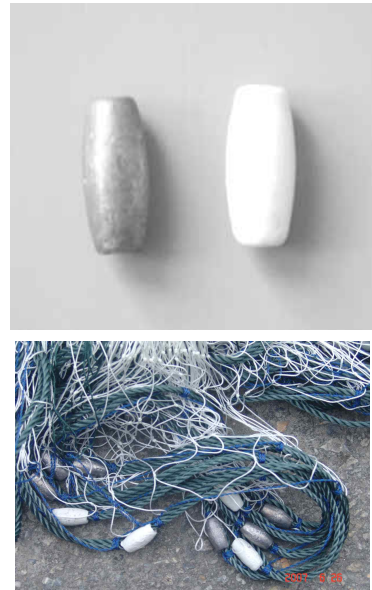
[Fig. 3] Coated sinker, lead sinker and experimental gill net
