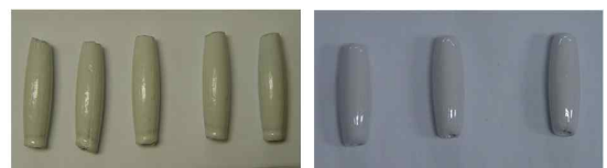
(a) Dried lead sinker in normal temperature (b) Dried lead sinker in the oven(100℃)
