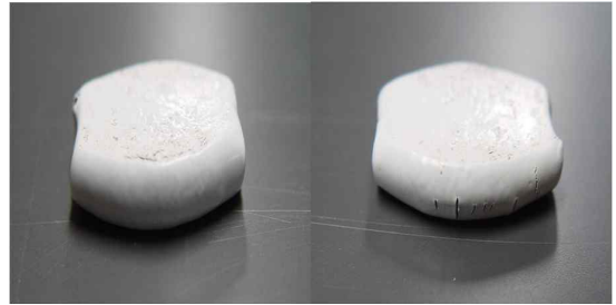
[Fig. 9] Durability test of coated sinker by press machine
