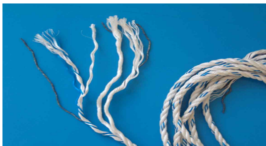
[Fig. 11] Lead line of ground rope for gill net
