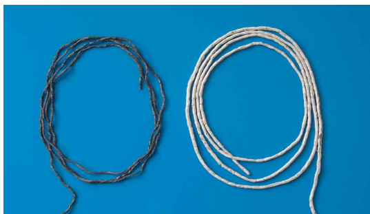
[Fig. 12] Lead line and coated lead line of ground rope for gill net
