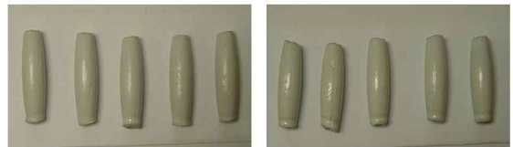
(a) 80wt% main materials + 20wt% thinner (b) 70wt% main materials + 30wt% thinner
