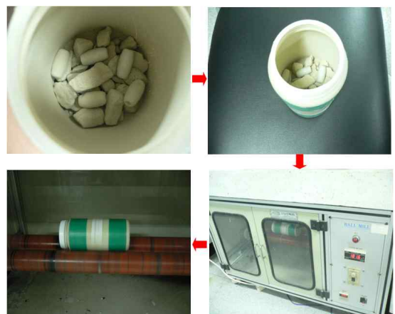
[Fig. 1] Process of abrasion test for the coated lead sinker
