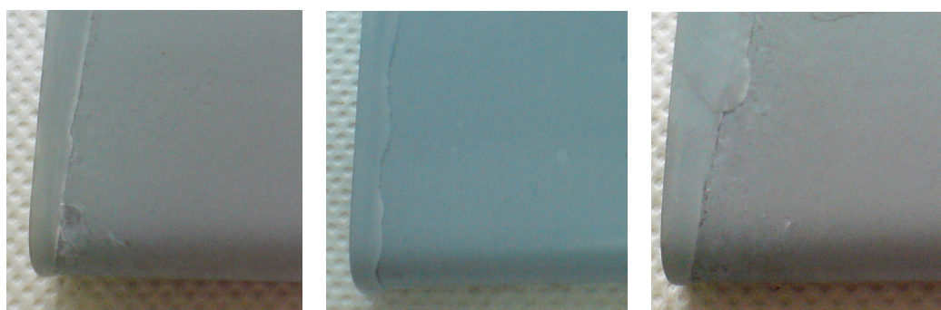
Fig. 7. Coated steel samples after bending test (180°, 8 mm mandrel) and subsequent neutral salt spray test (48 h), left: unmodified polymer resin, middle: resin with 10 wt.% unmodified silica, right: resin with 20 wt.% organo silane modified silica as representative samples.
