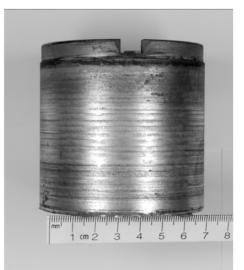
**Fig. 2.** The surface smoothness of the SiAlON blocks and the WC-coated 316L SS sleeve has been noticeably improved following a laboratory test, owing to the grinding/polishing effect induced by the sliding contact in the test.
