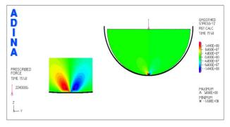
Fig. 1b. Shear stress  $\sigma_{yz}$  in the sleeve and shaft of an industry bearing with a radial clearance of 10 mm.
