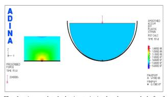
Fig. 1a. Accumulated plastic strain in the sleeve and shaft of an industry bearing with a radial clearance of 10 mm.
