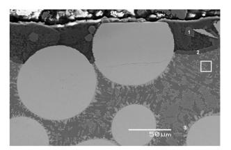
Fig. 3. Cross-section of a WC-coated 316L SS sleeve after being tested against a SiAlON bushing in a GL bath. The binder of the coating corroded severely, and its support of the WC particles was weakened. A transverse crack developed within the carbide slightly ahead of the advancing corrosion front in the coating. The particle (1) and the intermetallic layer forming at the corrosion front (2) are both of the  $\tau_5$  composition.
