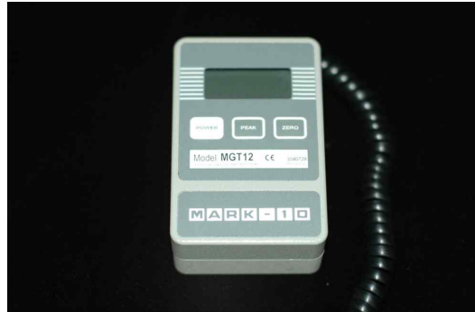
Fig. 4. Digital torque meter (MGT 12; Mark-10 Corp., NY, USA).
