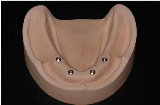
Fig. 2. Experimental stone cast with 4 external hexagon implant replicas made from acrylic resin splinted impression.
