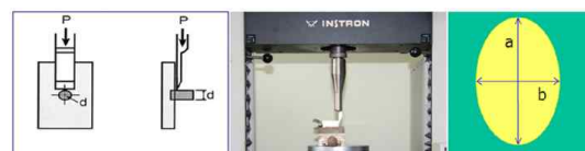
Fig. 4. Shear bond strength test in Universal testing mashine.
