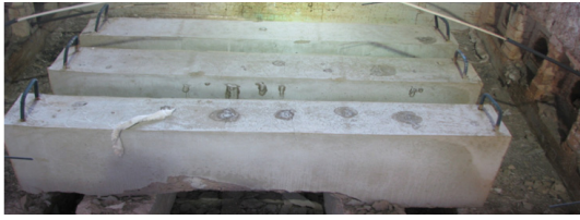
Fig. 10 Damaged specimens after fire test
