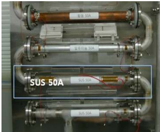
Fig. 2 Testbed for pipeline damage detection experiment
