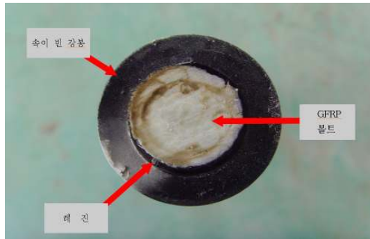
Fig. 2 Shape of GFRP rock bolt the inside
