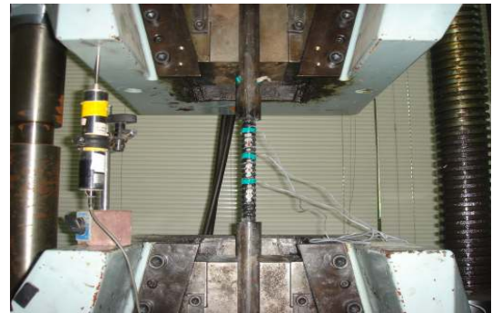
Fig. 4 Tension test of GFRP rock bolt
