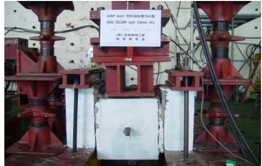
Fig. 15 Shear test result of GFRP rock bolt
