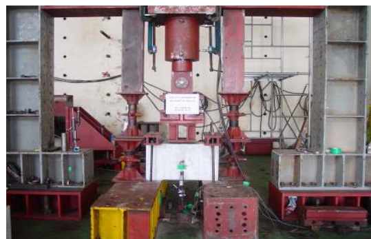
Fig. 9 Shear test of GFRP rock bolt
