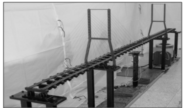
(a) Model Bridge for Vibration Control Tests
