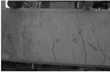
(a) Crack of Control specimen
