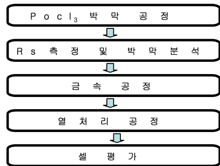
Figure 2. Process flow chart of silicon solar cell.
