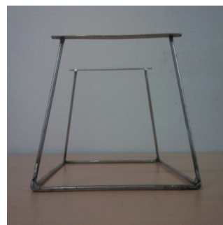
Fig. 1. mobile X-ray unit collimator Shielding device
