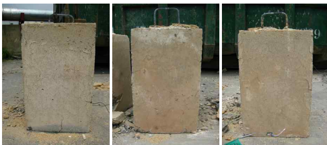
Figure 17. Appearance of specimens after fire test at series III
