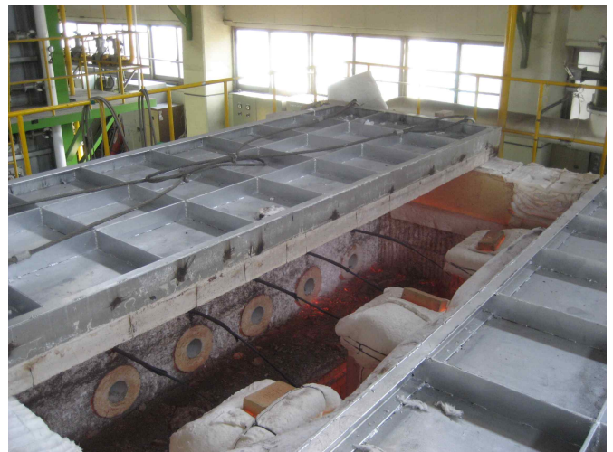
Figure 1. Fire test of high strength concrete
