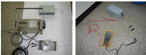
Figure 8. Half-cell potential & Corrosion current density measurement
