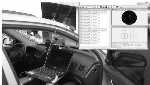
(a) GPS 수집장치 (a) GPS-equipped probe vehicle
